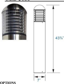
Formed 316 stainless steel housing with flush Mounting Base and Vandal-Resistant Screws, Domed Top. Internal Ballast Tray for Easy Maintenance. Cast Aluminum Louvers. Clear Polycarbonate Lens. Mounting Kit with 8" Anchor Bolts (Included). LED Array 14.5w, System 17w. Ideal for lighting pedestrian walkways and accenting the exterior grounds of office and apartment buildings, hotel and parks. Comes with a 5 year/50,000 hour limited warranty.
