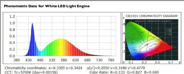
CCT: Tc=5700K (duv=0.00156) Color Ratio: R=0.133 G: Peak Wavelength: 447.2nm Half Bandwidth: 19.1nm Dominant Wavelength: 535.2nm Color Purity: 0.020 Color Render Index: Ra= 75.0,  $avgR(1\sim14)=65.6$ ,  $avgR(1\sim15)=65.9$
