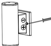
2. Use tools to unscrew both sides and remove mounting plates.
