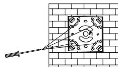
3. Fix the mounting plate to the junction box with the screwdriver
