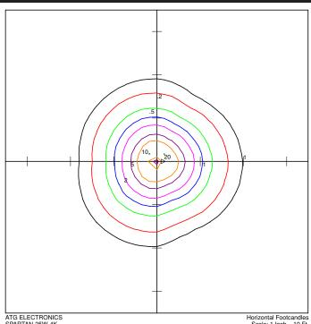
ATG ELECTRONICS SPARTAN-25W-4K 8" DIAM. X 42" HEIGHT, LED BOLLARD LED MODULE WITH POLYCARBONATE Horizontal Footcandles
