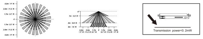
NOTE: The high-frequency output of this sensor is <0.2mW - that is just one 5000th of the transmission power of a mobiel phone or the output of a microwave oven.
