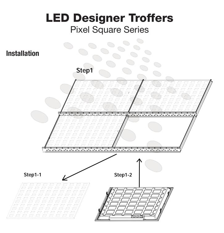
Step 1: Make sure of all the power is off before installing. Remove the one ceiling tile that you need to install light fixture on. Then place the light fixture on the T-bar carefully and make sure it is correctly in place and secure.
