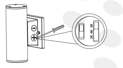
Note:Please turn off the power before adjusting the wattage and CCT. CCT adjustable instruction fixture.
