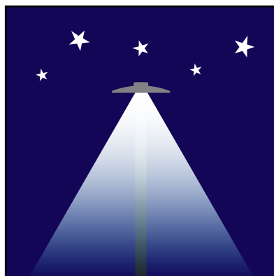
The CESP is a complete cutoff, fully shielded area light that minimizes glare, while reducing light trespass. (The maximum luminous beam angle 90°)
