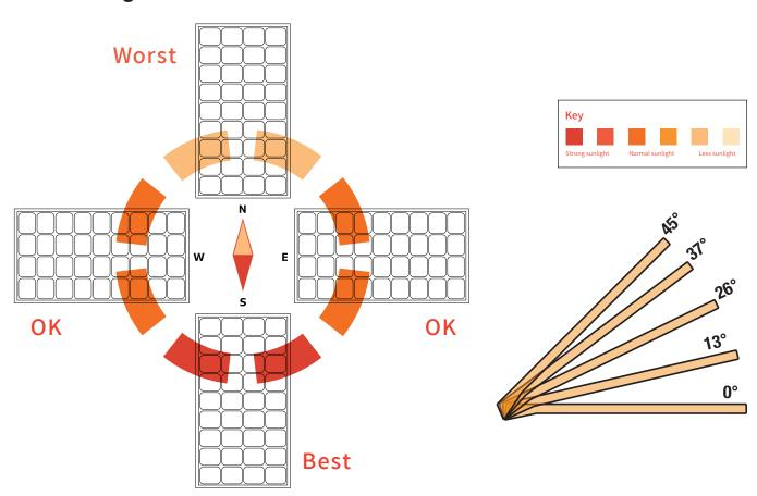
The area will dictate the installation of the fixtures and will sometimes prevent the lights from facing south. Panels facing West & East won't get as much light as Southern facing panels, but will stillcollect a good amount of sunlight. A North facing panel also works, but it will take longer to charge than any other direction. This would mean that the solar charge will be less optimal if installations are facing North.
