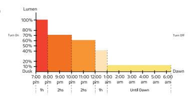
Changes as natural light decreases/increases (turns on at dusk); 100% brightness for 1 hour, 70% brightness for 2 hours, 60% brightness for 2 hours, 40% brightness for 1 hour, 100% brightness for the rest of the night (turns off at Dawn).
