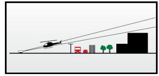
Under these conditions ICAO Annex 14 Vol.II recommends the helipad to be complemented with the aid of Visual approach slope indicator System.
