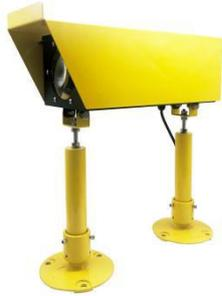
The LED CHAPI Heliport Approach Path Indicators (CHAPI) uses LED technology to provide the pilot with safe and accurate glide slope on final approach to the helipad. A set of two LED CHAPI Light Housing Assemblies (LHAs) are seen by the pilot in combinations of white, green and red to indicate a path that is too high, too low or within the  $6^\circ \pm 0^\circ 15'$  glide slope.
