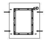
**Step 4**: Screw and fasten the PC frame back to the light with one screw on the top and two screws at the bottom.
