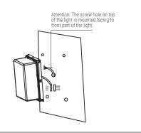
**Step 3**: Screw and fasten the light to the wall with 4 KA5X12 screws on the 4 corners of the light.
