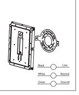
Step 5: Screw and fasten the light on the bracket with screws on both sides of the lights.
