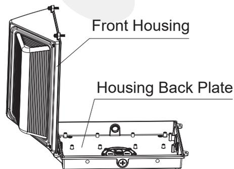
5. The bottom shell is sprayed with glue and tightly sealed to the wall. The fixture must be mounted on the wall with the lens facing down as shown in the picture. After the product is installed, remove the two drain hole plugs to prevent internal water accumulation.
