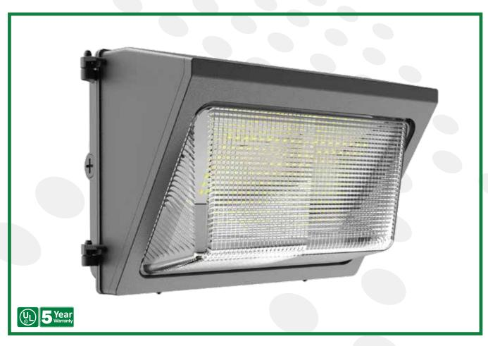
Beyond LED's FORTE wall pack is the newest, most innovative and feature rich product of 2023. It offers 4 Adjustable wattages and 3 Adjustable CCT with energy-efficient LED technology. FORTE comes with Built-in photocell. FORTE luminaires comes with die cast aluminum housing and glass lens to stand up for many years of punishing environmental conditions.
